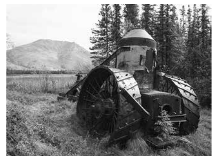
Upper image: Edward Kindle of the U.S. Geological Survey poses next to the 110-horsepower Best traction engine along the Yukon River, 1906. USGS Photographic Library, Edward Kindle (107). Lower image: The Best traction engine a century later, stripped of its cabin and boiler chimney. Photo by Todd Croteau of the Historic American Engineering Record.
