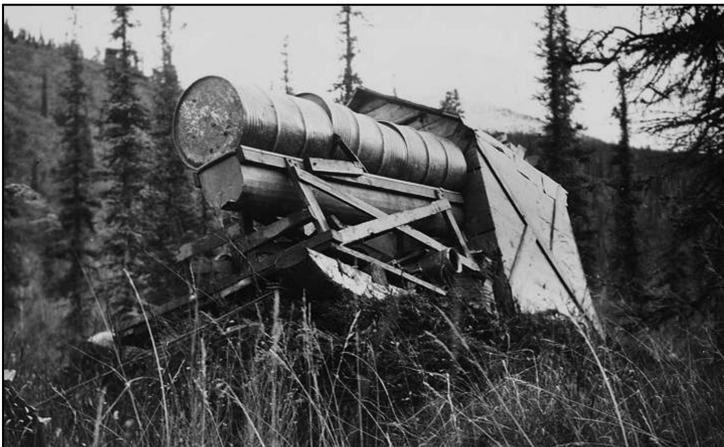
A Caterpillar tractor pulled this "go-devil," a sled that carried supplies for the "Prospector" churn drill. The sled carried fuel, tools, bits, drill pipe, and steel sluice boxes for processing the rock slurry recovered from drill holes. (SP)
